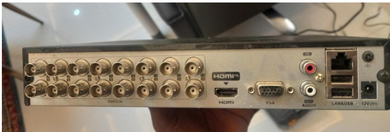
FIG 15: CONNECTION PORTS FOR DIGITAL VIDEO RECORDER (DVR)
