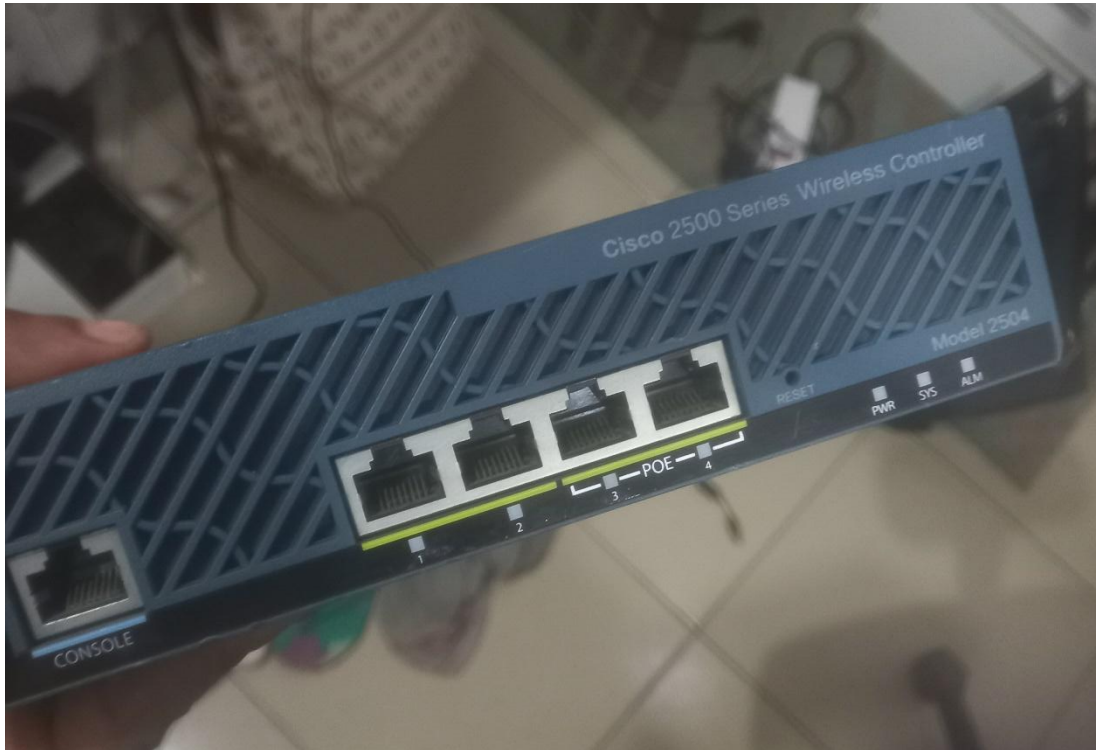
FIG 5: TESTING A CISCO WIRELESS CONTROLLER
